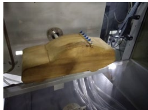
Fig.12: Vehicle with Parabolic VG in Wind Tunnel
