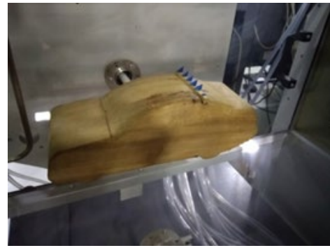
Fig.11: Vehicle with Triangular VG in Wind Tunnel
