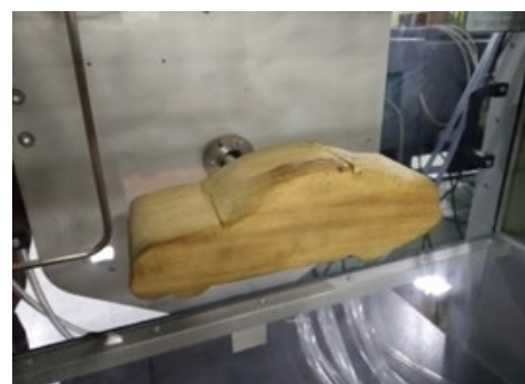
Fig.13: Vehicle without VG in Wind Tunnel
